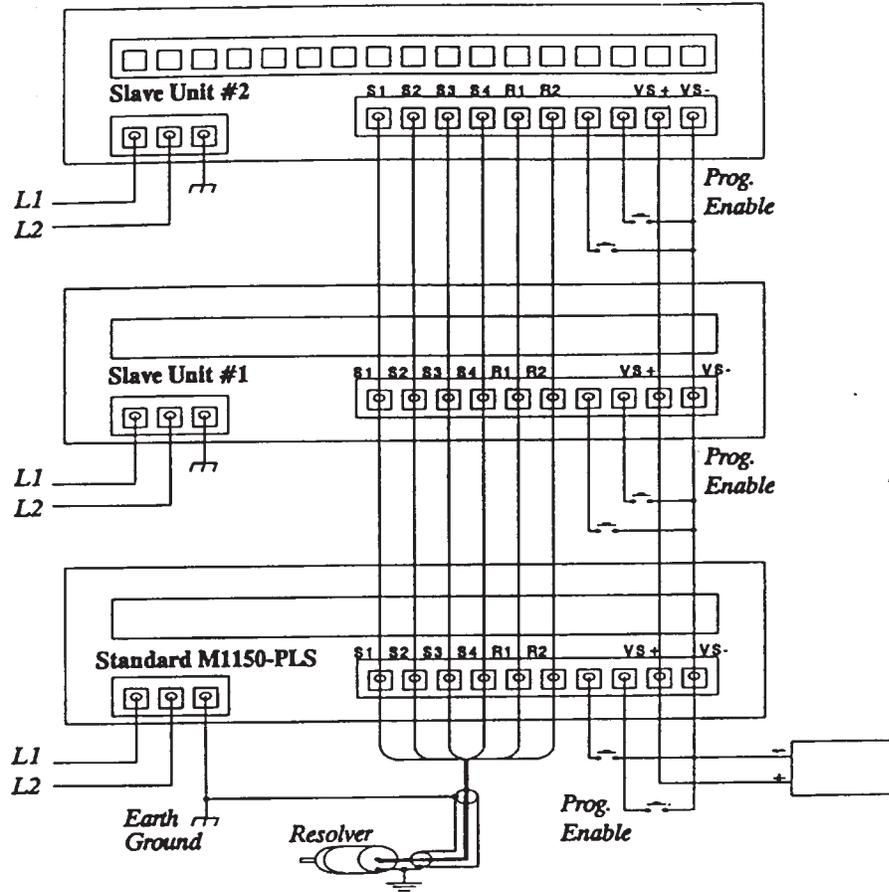
Slave M1150 units are special factory supplied M1150 units. DO NOT attempt to slave together two standard M1150 units — improper operation will result.
