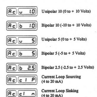
Press MODE key to save the displayed option, and to advance to Offset Calibration Mode.
