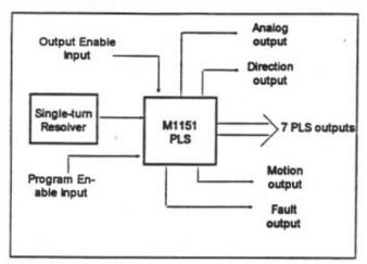
The M1151 programmable limit switch (PLS) uses a resolver, such as Autotech's RL100, E6R, E7R or E8R series of resolvers, as a position transducer. The M1151 PLS controls 7 or 15 PLS outputs (turns ON/ OFF), according to the programmed position limits for each ouput. The M1151 also offers a motion output, which energizes when the resolver is rotating at a speed within the programmed motion limits.
