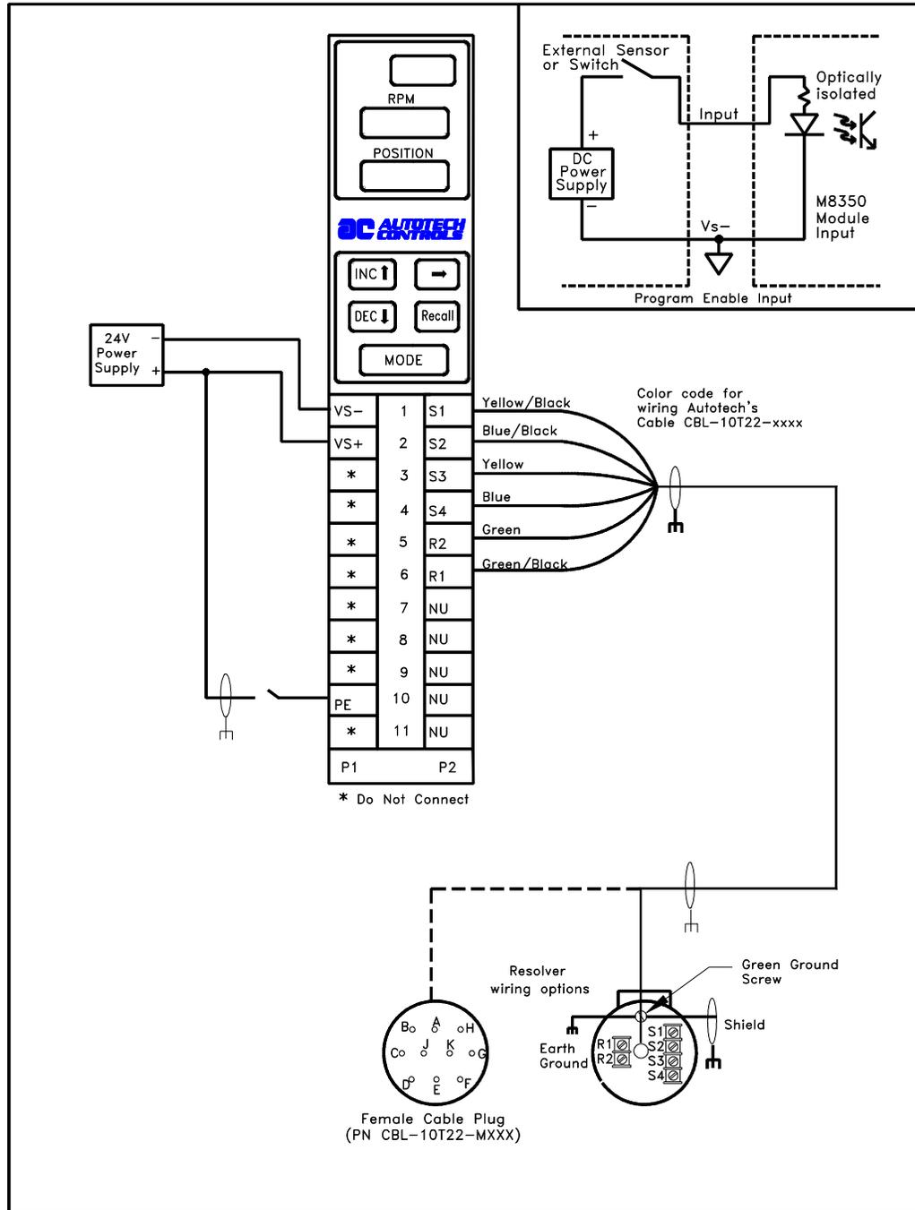
Figure 3. M8350-010 Wiring Diagram
